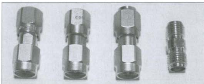
Figure 10: The 'Poor Man's Calibration Kit'. From left to right we see Open, Short, Load and Through.
