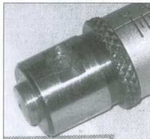
Fig. 14: Milled cut for counter screw
