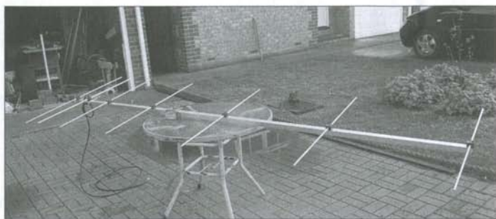
Fig. 10: The finished antenna before installation on the tower. Note the very close spacing of the first three elements, the visible characteristic of the OWL antenna
