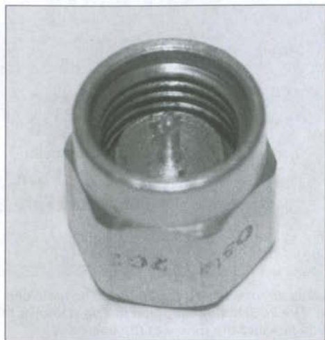
Figure 9: On the left, a standard SMA short. This is screwed onto the same Radial adapter as Figure 7. On the right is the cross-section through the simulation setup (only the metal disc and the centre pin need to be modelled).
