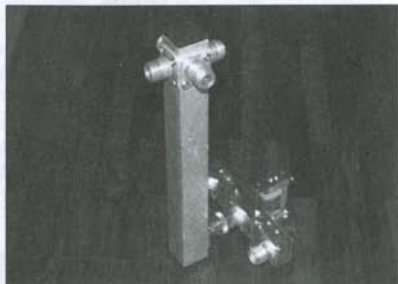
Fig. 11: 4 port splitter directly connected to HF 400 coaxial relay
